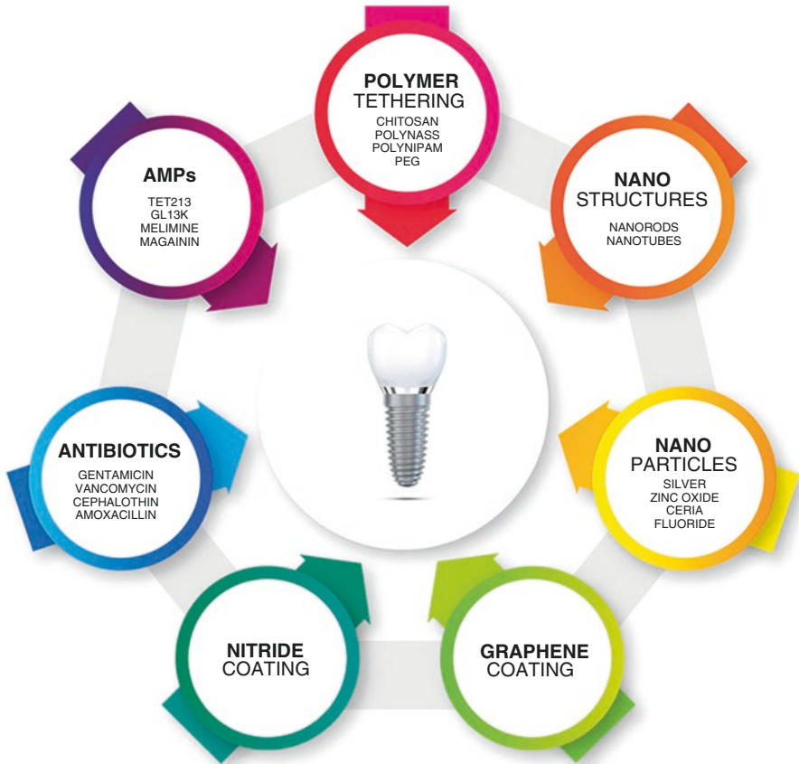
Fig. 9.6 Strategies for controlling biofilm on dental implants in the modern era (Sivaswamy and Neelakantan 2022)
